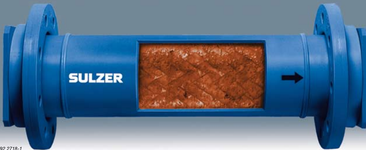
Figure 11: SMO 2 mixer in polypropylene for the aeration of water in the oxidation process for iron and manganese removal.
