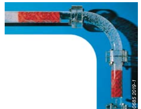
Figure 4: Bubble bed with vertical and horizontal Sulzer mixer SMV-12 NPS 50 mm and phase separation in the horizontal empty pipe. System air/water. Flow velocity 0.5 m/s.
