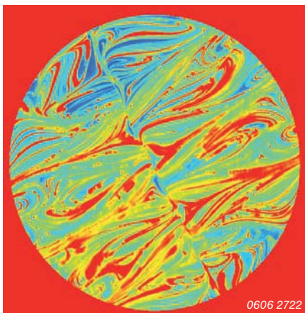
Laminar mixing in the Sulzer SMX™ mixer shown with Laser Induced Fluorescence
