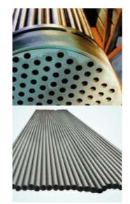
Our graphite tubes are manufactured in France by an extrusion process which produces up to 6 meter long tubes without a joint. The tubes have the highest mechanical resistance (G30-00-220) certified by TÜV.
