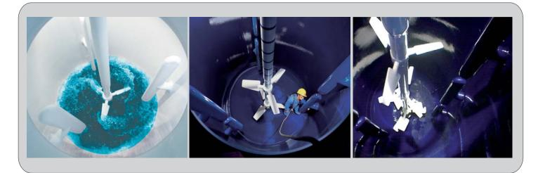
Depending on their capacity, our OptiMix<sup>®</sup> reactors are fitted with 1 to 3 rows of 3 baffles welded to the wall.
