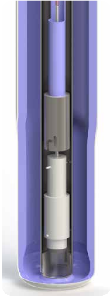
Assembly of a DR probe in a baffle
