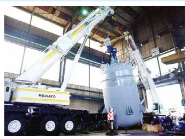
King size glass-lined reactor Handling 75 tonnes
