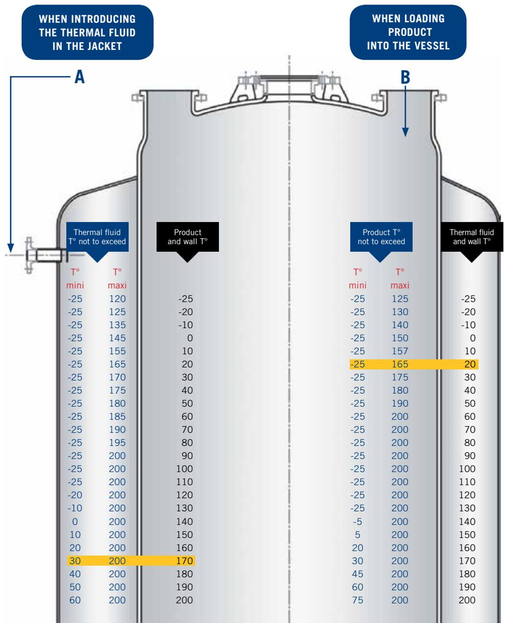
The maximum  $\Delta T$  values given in these tables MUST be respected. They are limit values which must not be exceeded.
